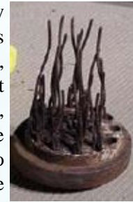
Severe corrosion of strands within about two decades; Good grouting can prevent this.
