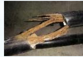
Severe corrosion of strands within about two decades; Good grouting can prevent this.
